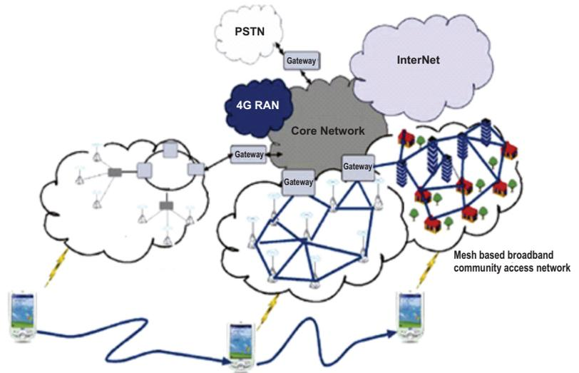
Figure 10 Mesh based topology
