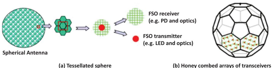
Figure 9 3-D spherical FSO systems tessellated with optical transceivers
