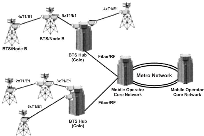
Figure 4 Backhaul connection through FSO
