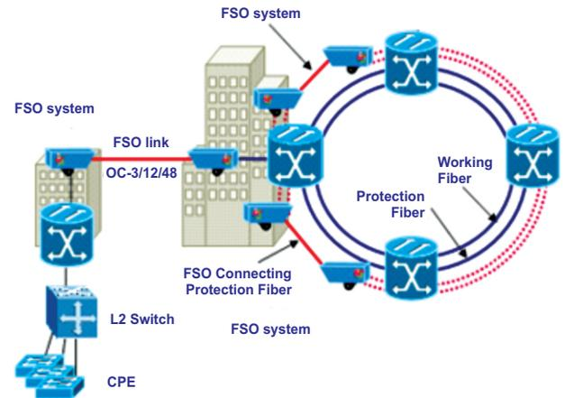
Figure 2 Network extension and fibre complement through FSO
