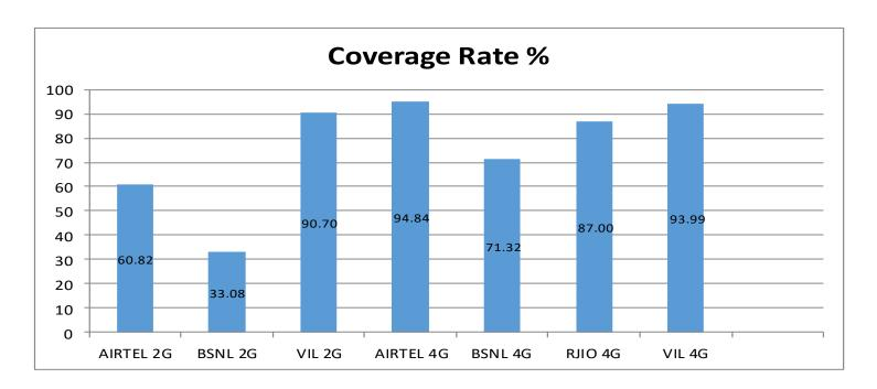
**Note- Coverage** is the percentage of samples having signal strength more than the threshold value ( $2G \ge -85$  dbm,  $3G \ge -90$  dbm and  $4G \ge -110$  dbm). However, these samples are only for the portion of the OADT routes where TSPs have coverage i.e 'no coverage' routes have been excluded.
