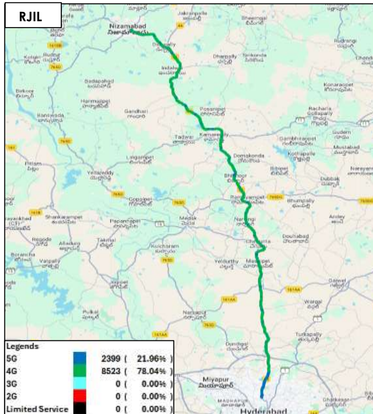
Figure-37: Serving technology plots in auto-selection mode (5G/4G/3G/2G)-RJIL.
