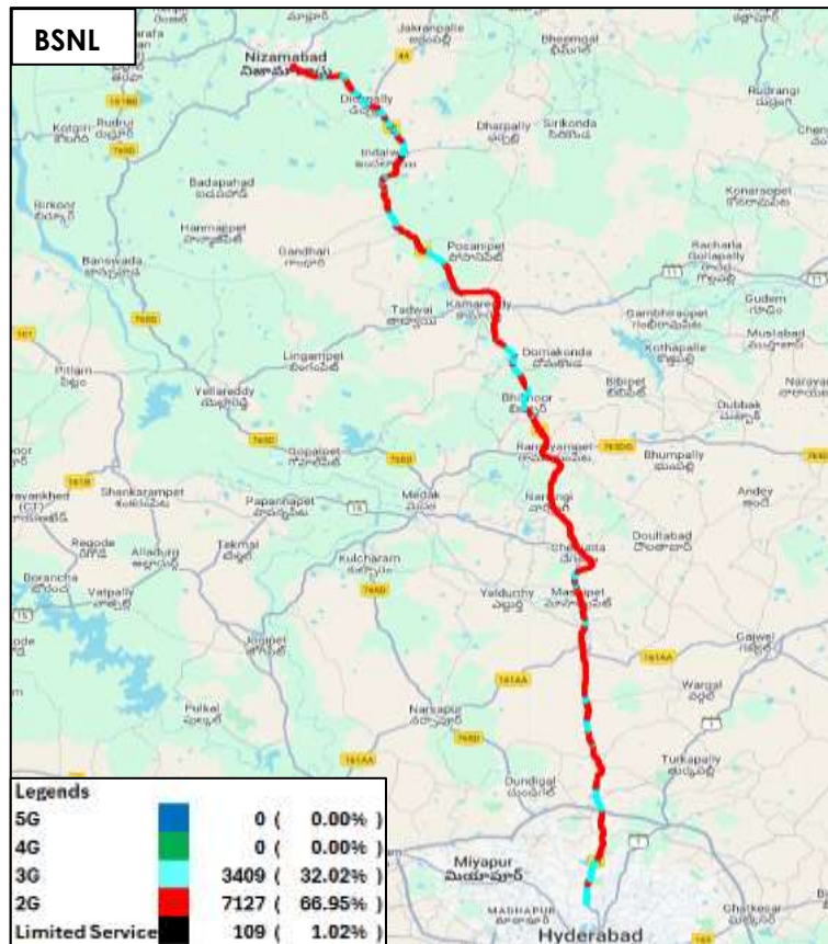
Figure-36: Serving technology plots in auto-selection mode (5G/4G/3G/2G)-BSNL.
