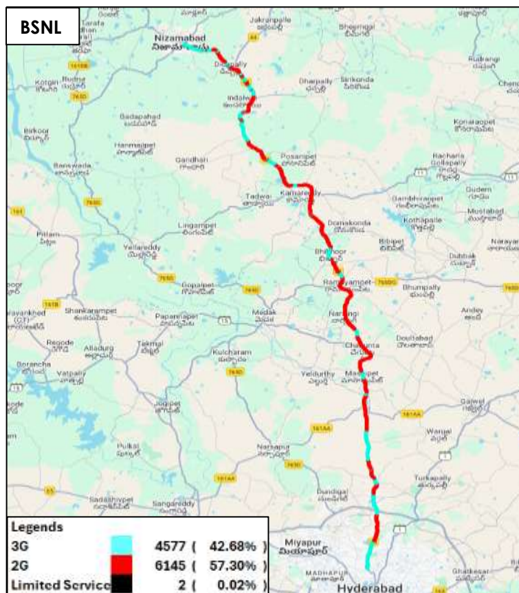
Figure29: Serving technology plots 3G/2G network mode – BSNL.
