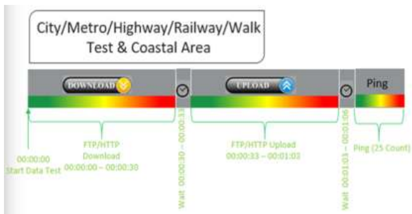
Figure-60: Data test script used in city/metro/railway/highway/walk test & coastal area
