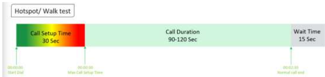
Figure-59: Voice test script for walktest/hotspot
