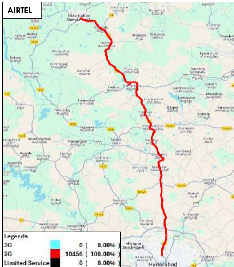
Figure-28: Serving technology plots 3G/2G network mode – AIRTEL.
