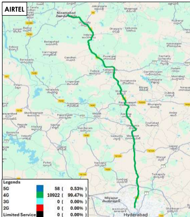
Figure-35: Serving technology plots in auto-selection mode (5G/4G/3G/2G)-AIRTEL
