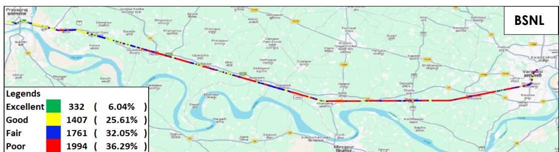
Figure-61: Signal strength auto-selection mode (5G/4G/3G/2G) data - BSNL.
