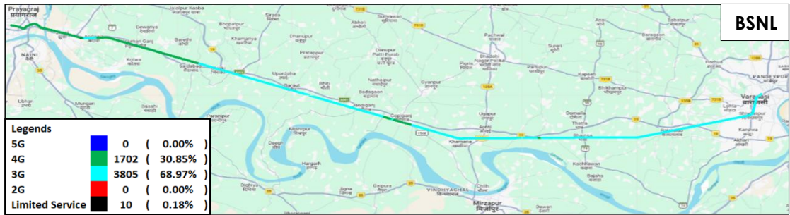
Figure-41: Serving technology plot in auto-selection mode (5G/4G/3G/2G) data - BSNL.
