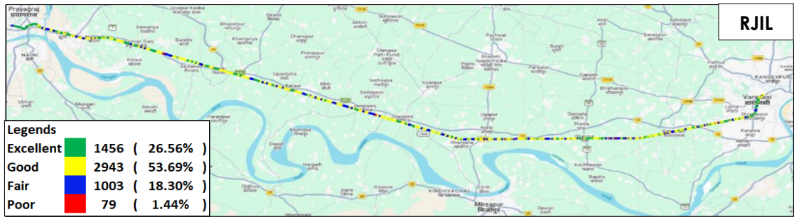
Figure-58: Signal strength auto-selection mode (5G/4G/3G/2G) voice - RJIL.
