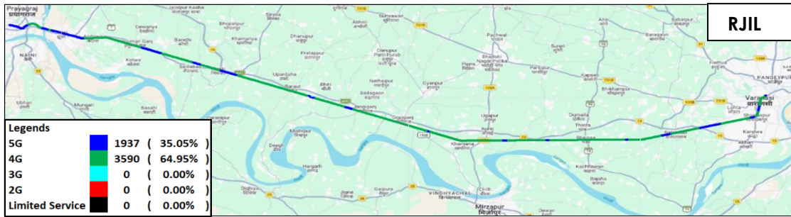
Figure-35: Serving technology plots in auto-selection mode (5G/4G/3G/2G) voice - RJIL.
