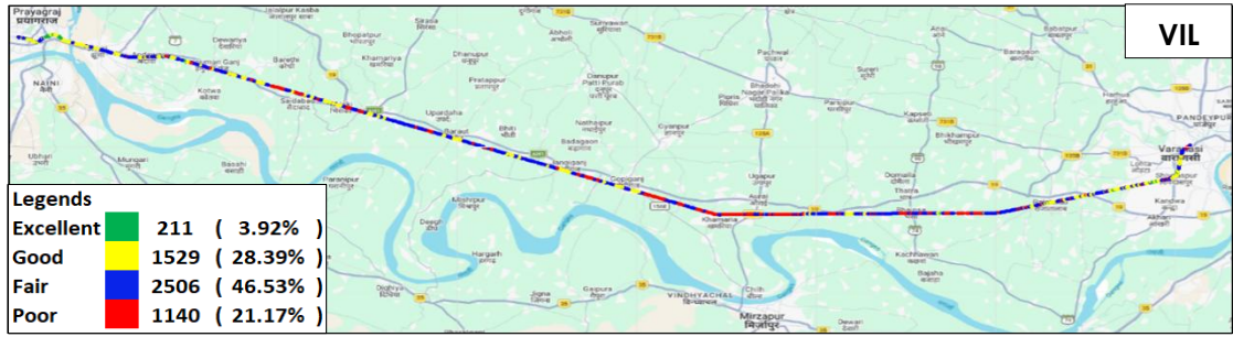
Figure-63: Signal strength auto-selection mode (5G/4G/3G/2G) data - VIL.
