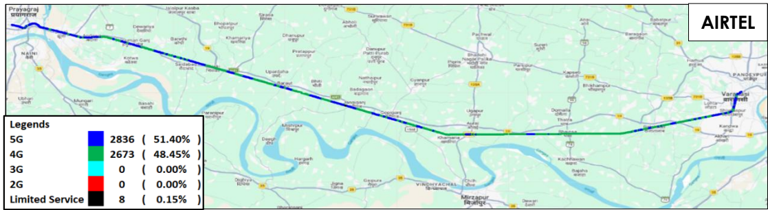
Figure-40: Serving technology plot in auto-selection mode (5G/4G/3G/2G) data - AIRTEL.
