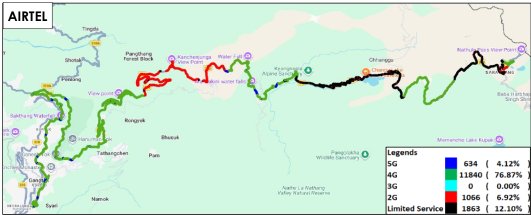
Figure-39: Serving technology plots in auto-selection mode (5G/4G/3G/2G) voice – AIRTEL.
