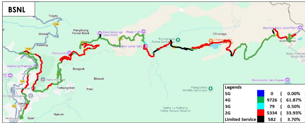
Figure-40: Serving technology plots in auto-selection mode (5G/4G/3G/2G) voice - BSNL.
