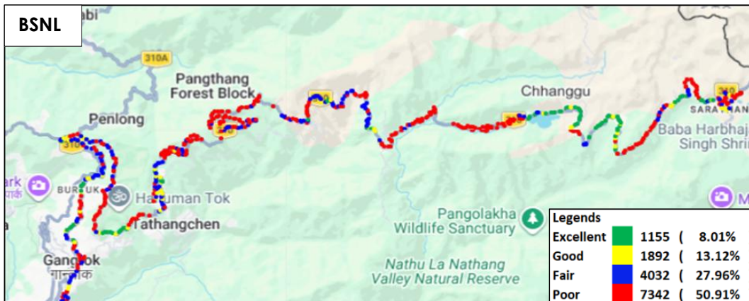
Figure-63: Signal strength 3G/2G network mode voice - BSNL.
