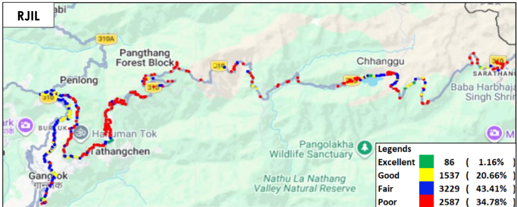
Figure-71: Signal strength auto-selection mode (5G/4G/3G/2G) data - RJIL.
