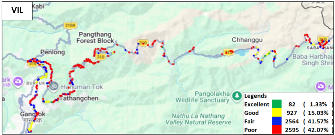
Figure-72: Signal strength auto-selection mode (5G/4G/3G/2G) data - VIL.
