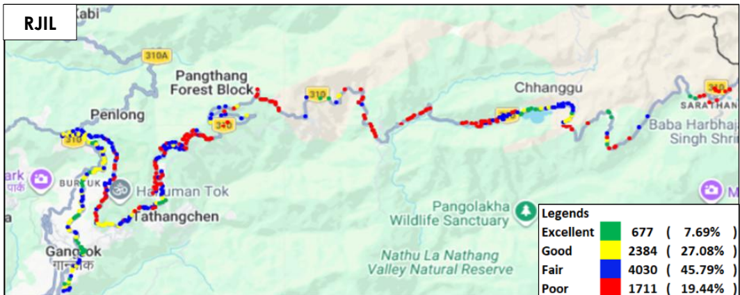
Figure-67: Signal strength auto-selection mode (5G/4G/3G/2G) voice - RJIL.
