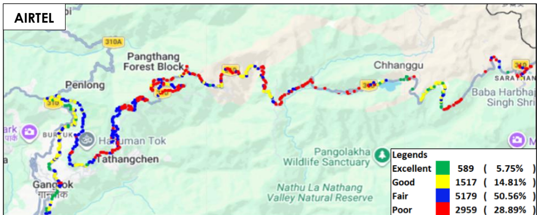
Figure-69: Signal strength auto-selection mode (5G/4G/3G/2G) data - AIRTEL.
