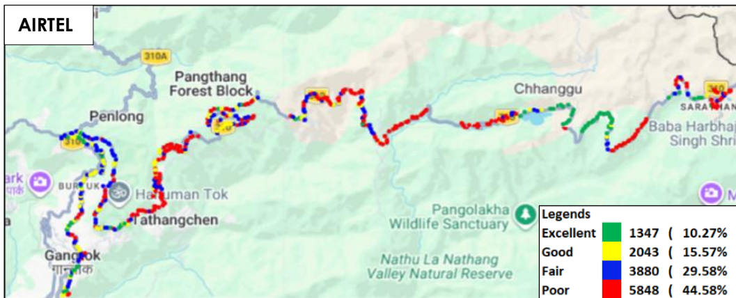
Figure-62: Signal strength 3G/2G network mode voice - AIRTEL.
