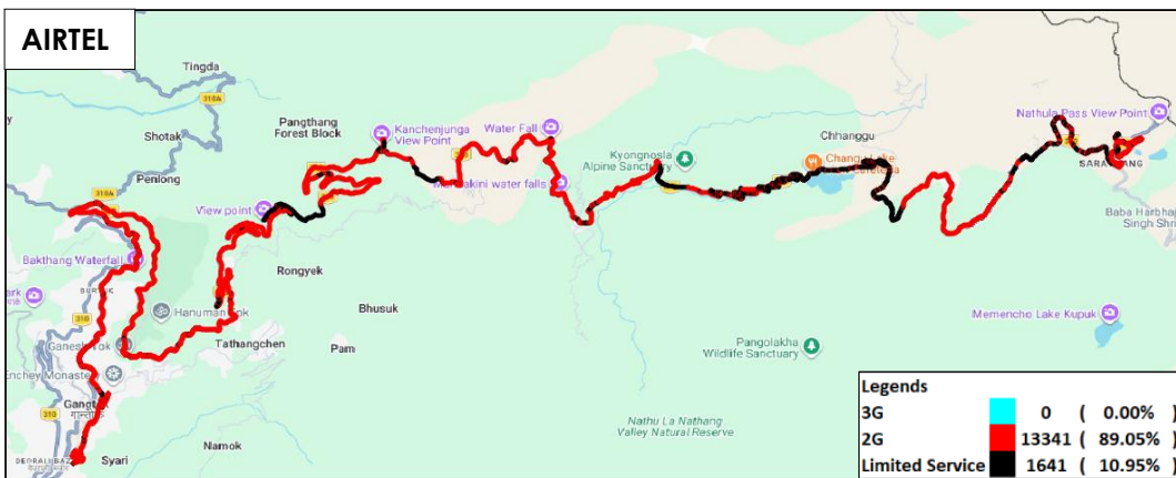
Figure-32: Serving technology plots 3G/2G network mode - AIRTEL.
