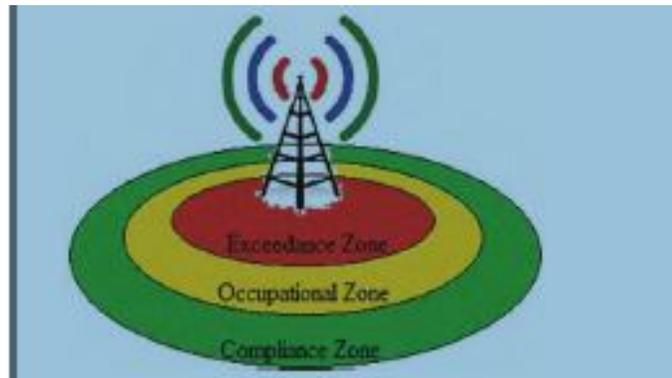
For distances greater than the compliance zone, the radiation levels are under limits. Compliance zone indicates a safe distance from the antennae. In the compliance zone, potential exposure to EMF is below the applicable limits as shown in figure 1.9 above.
