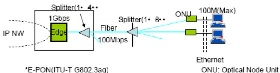
**Fig 24: Sharing a fibre, with a LAN SW / VDSL installed in customers' premises**
