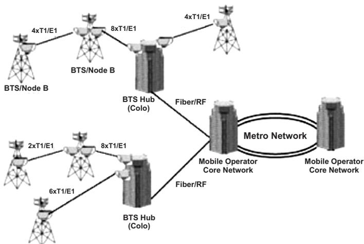
Figure 4 Backhaul connection through FSO
