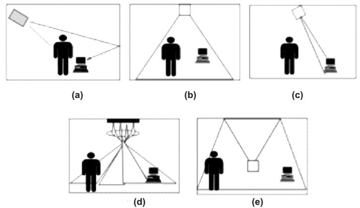
Figure 11 (a) Diffuse system. (b) Wide LOS system (c) Narrow LOS system with tracking (d) Narrow LOS system using multiple beams (e) Quasi diffuse system
