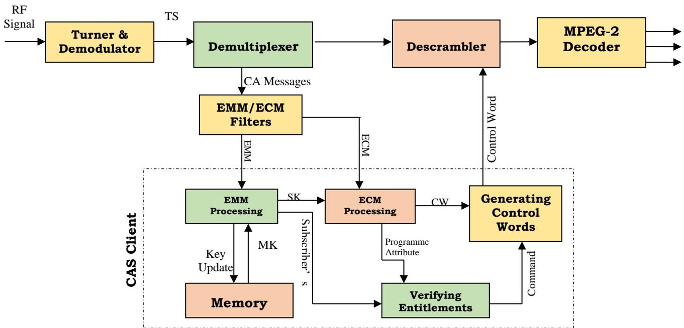
*Figure 9: Structure of CAS client at STB*
