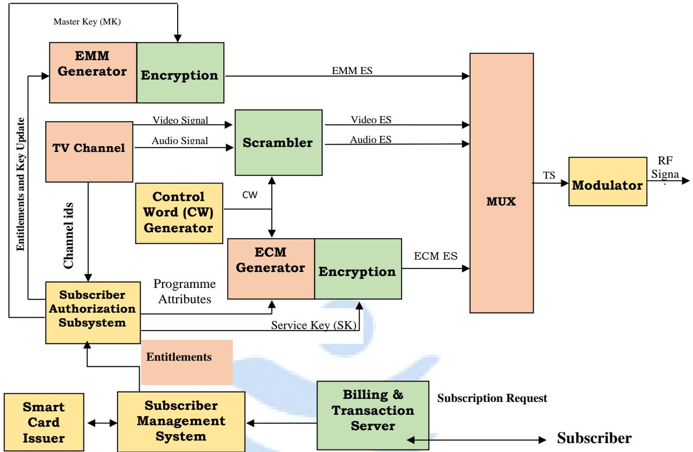
Figure 8: The basic structure of CAS at the transmitter side in an encrypted TV Broadcasting Service
