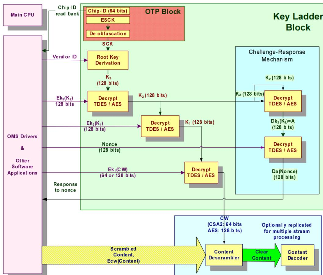
Figure 12: Key Ladder Block Diagram<sup>25</sup>
