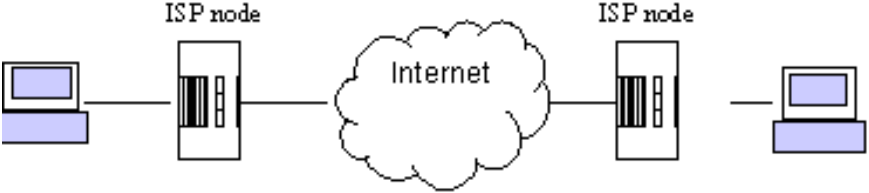
Fig 7: PC to PC communication for Internet telephony
