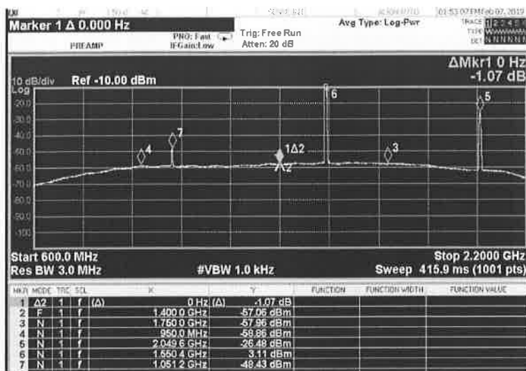
Figure 4. Output of a standard LNB with input CW
