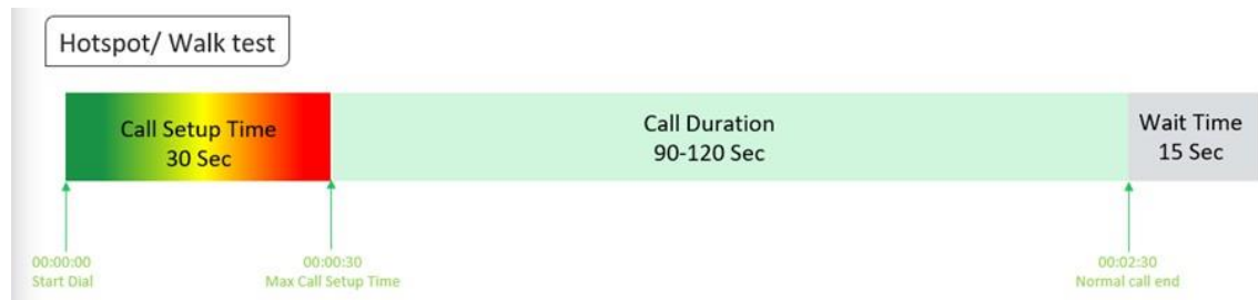
Figure-35: Voice test script for walktest/hotspot
