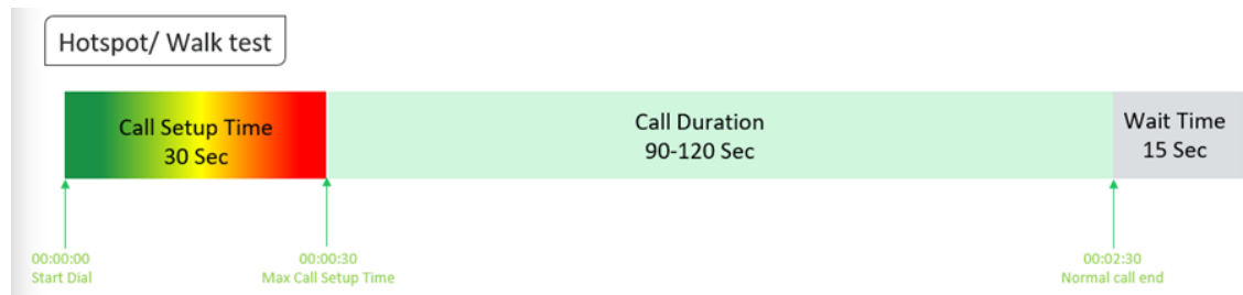
Figure-59: Voice test script for walktest/hotspot
