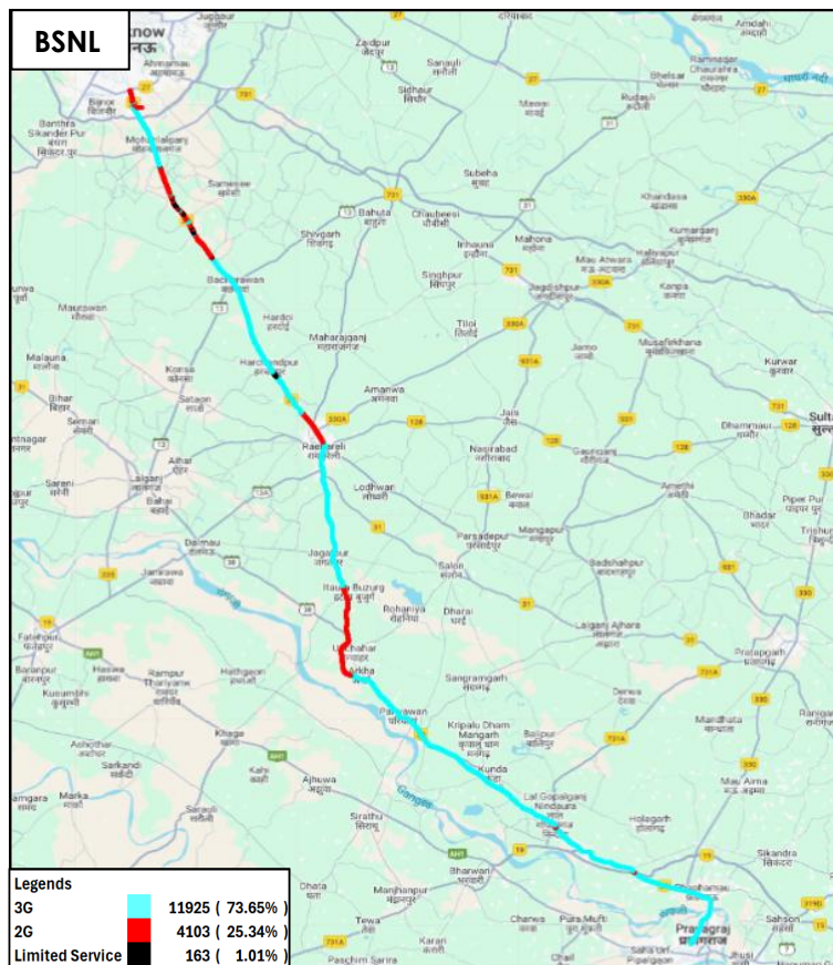
Figure29: Serving technology plots 3G/2G network mode – BSNL.
