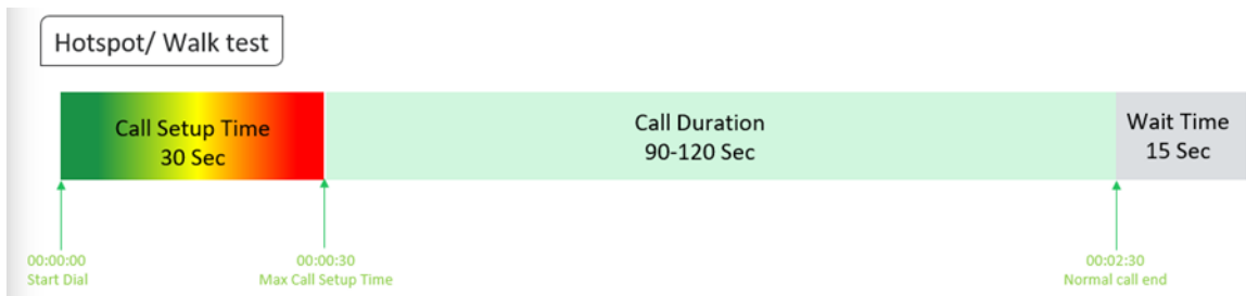
Figure-44: Voice test script for walktest/hotspot
