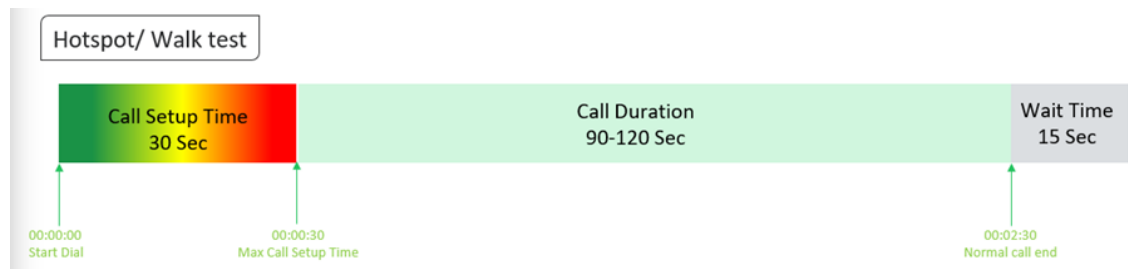
Figure-44: Voice test script for walktest/hotspot
