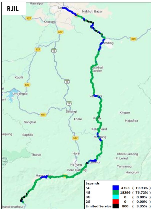
Figure-26: Serving technology plots in auto-selection mode (5G/4G/3G/2G) data - RJIL.
