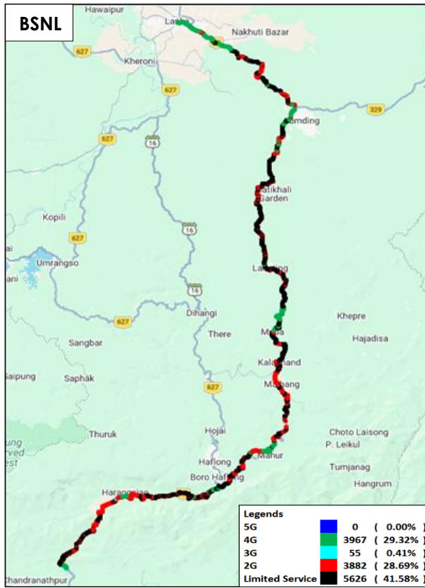
Figure-25: Serving technology plots in auto-selection mode (5G/4G/3G/2G) data - BSNL.
