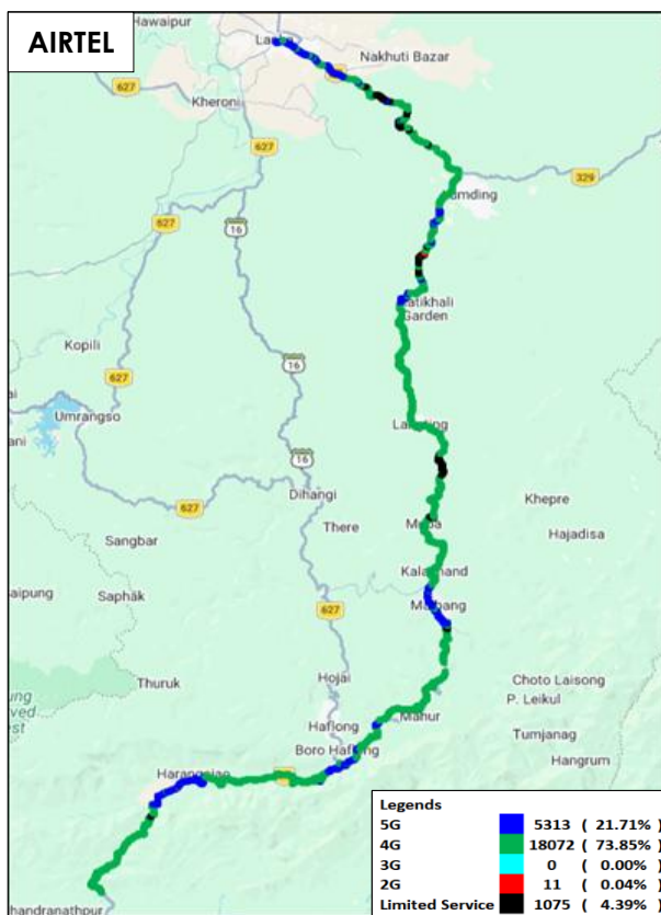
Figure-24: Serving technology plots in auto-selection mode (5G/4G/3G/2G) data - AIRTEL.
