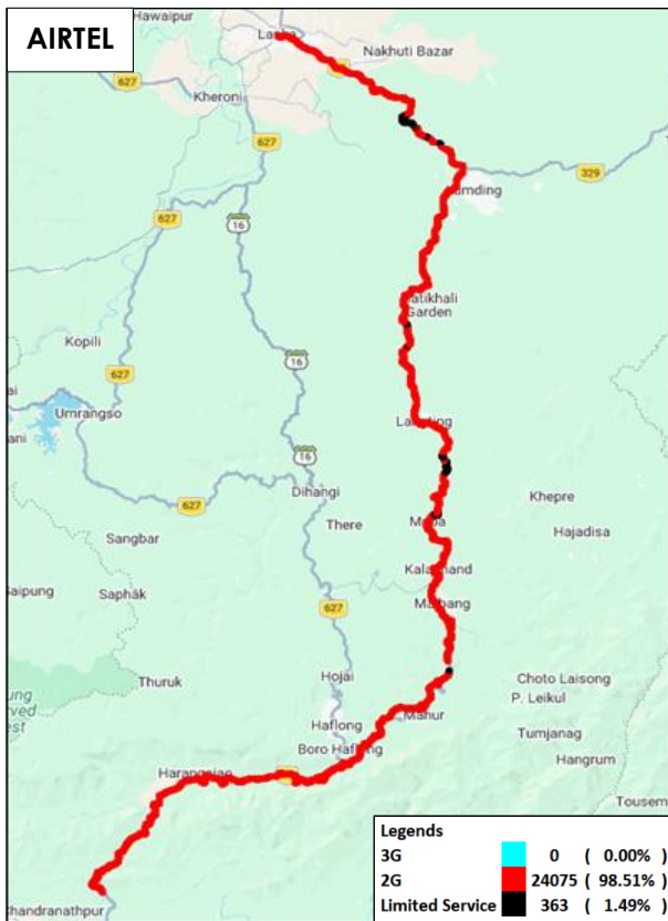
Figure-10: Serving technology plots 3G/2G network mode - AIRTEL
