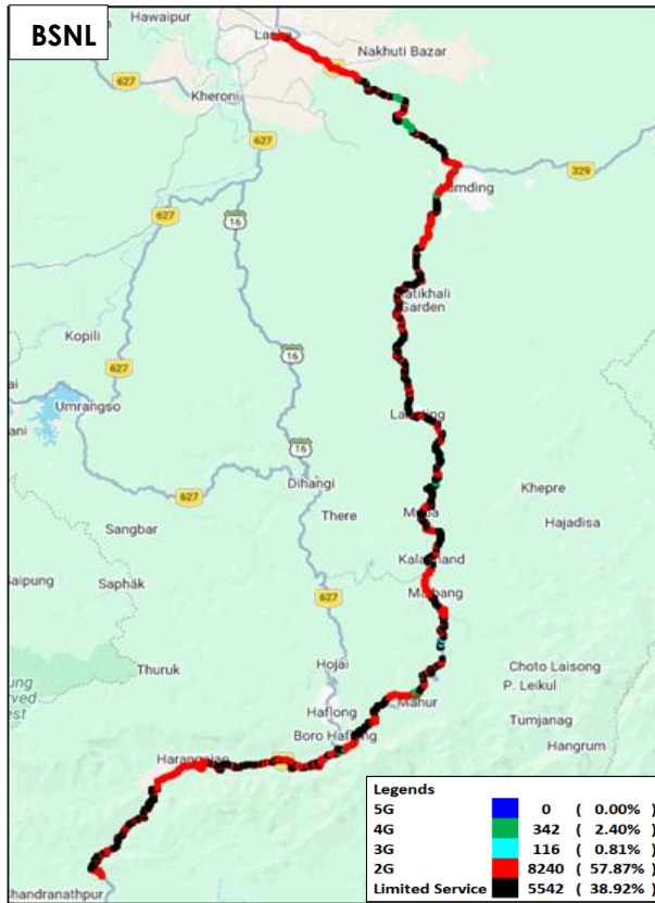
Figure-18: Serving technology plots in auto-selection mode (5G/4G/3G/2G) voice - BSNL.
