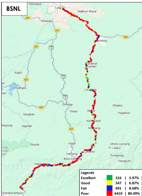
Figure-33: Signal strength auto-selection mode (5G/4G/3G/2G) voice - BSNL.
