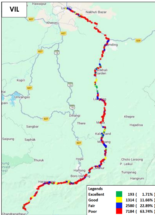
Figure-39: Signal strength auto-selection mode (5G/4G/3G/2G) data - VIL.
