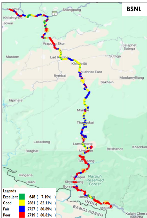
Figure-70: Signal strength auto-selection mode (5G/4G/3G/2G) voice - BSNL.
