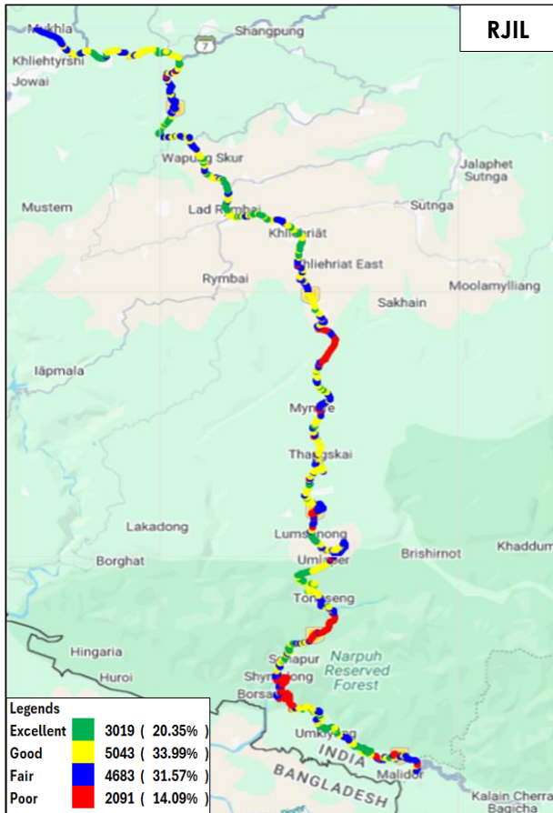
Figure-71: Signal strength auto-selection mode (5G/4G/3G/2G) voice - RJIL.
