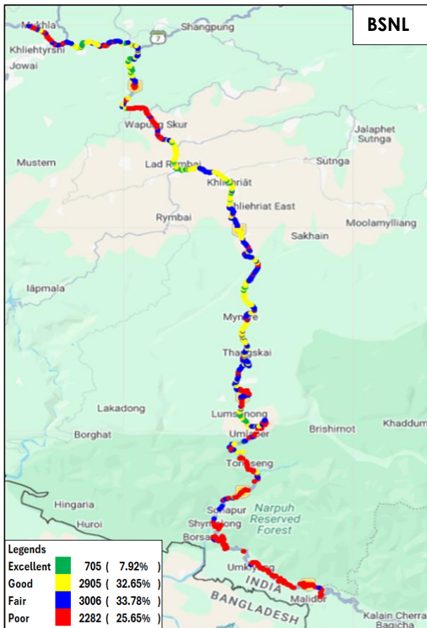
Figure-74: Signal strength auto-selection mode (5G/4G/3G/2G) data - BSNL.
