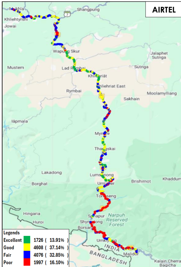
Figure-69: Signal strength auto-selection mode (5G/4G/3G/2G) voice - AIRTEL.
