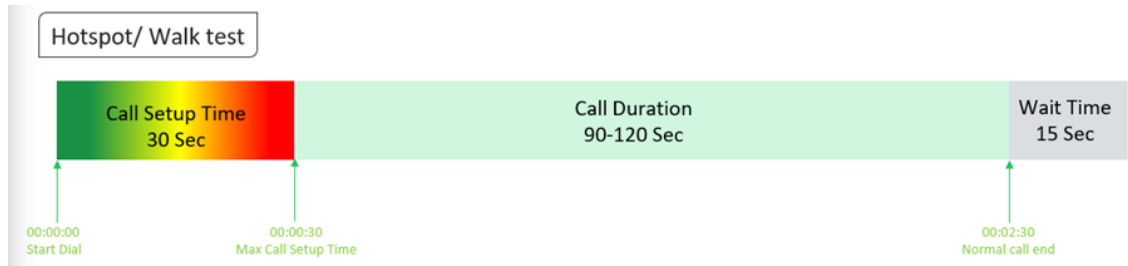
Figure-80: Voice test script for walktest/hotspot
