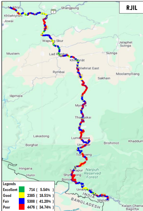
Figure-75: Signal strength auto-selection mode (5G/4G/3G/2G) data - RJIL.
