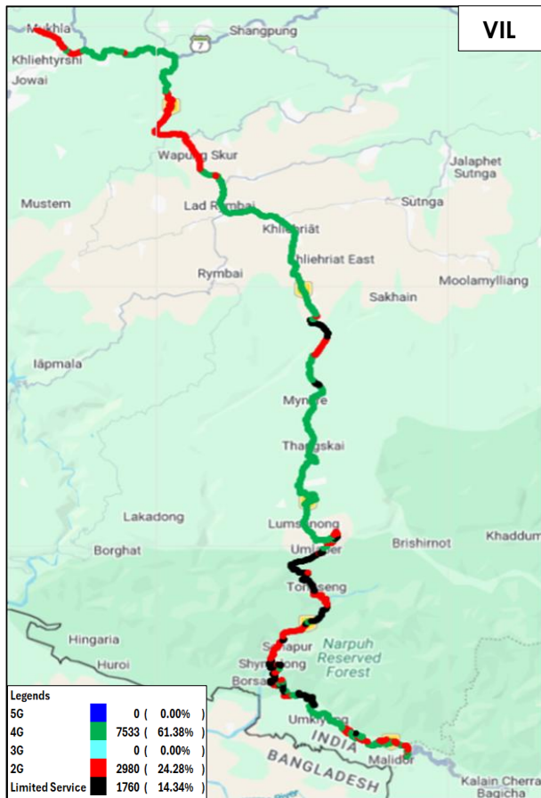
Figure-53: Serving technology plots in auto-selection mode (5G/4G/3G/2G) data - VIL.
