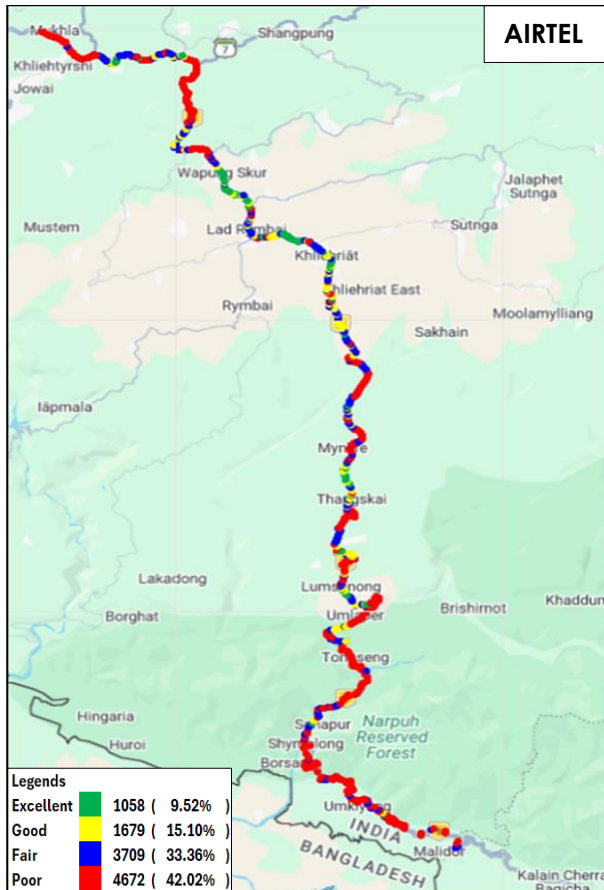
Figure-66: Signal strength 3G/2G network mode voice - AIRTEL.
