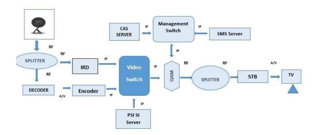
Figure 1.2: - Digital Headend System Block Diagram
