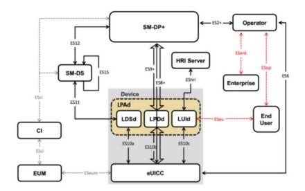
Figure: Remote SIM Provisioning for Consumer Architecture<sup>10</sup>
