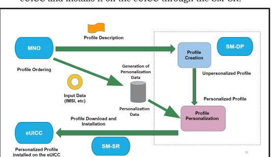
Operator. It finally builds Personalized Profiles for the targeted eUICC and installs it on the eUICC through the SM-SR.
