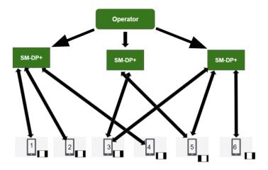
Figure: A Single Operator manages Multiple SM-DP+
