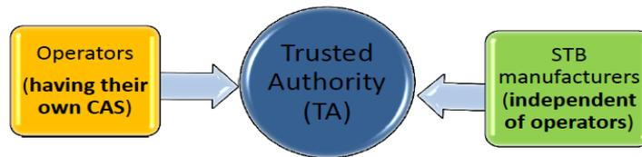
to the DPOs. STB manufacturers and DPOs would be required to apply for getting an authentication code from this nodal agency. Using these authentication codes, the STB manufacturer would fuse the STBs at the manufacturing stage with individual secure keys. These secure keys can serve as the STB identifier in a similar manner as to the IMEI numbers of mobile phone handset.
