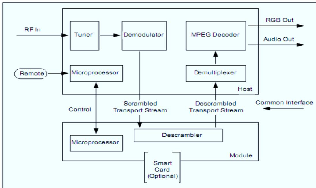
**Figure 7: Functional Block Diagram of a STB**
