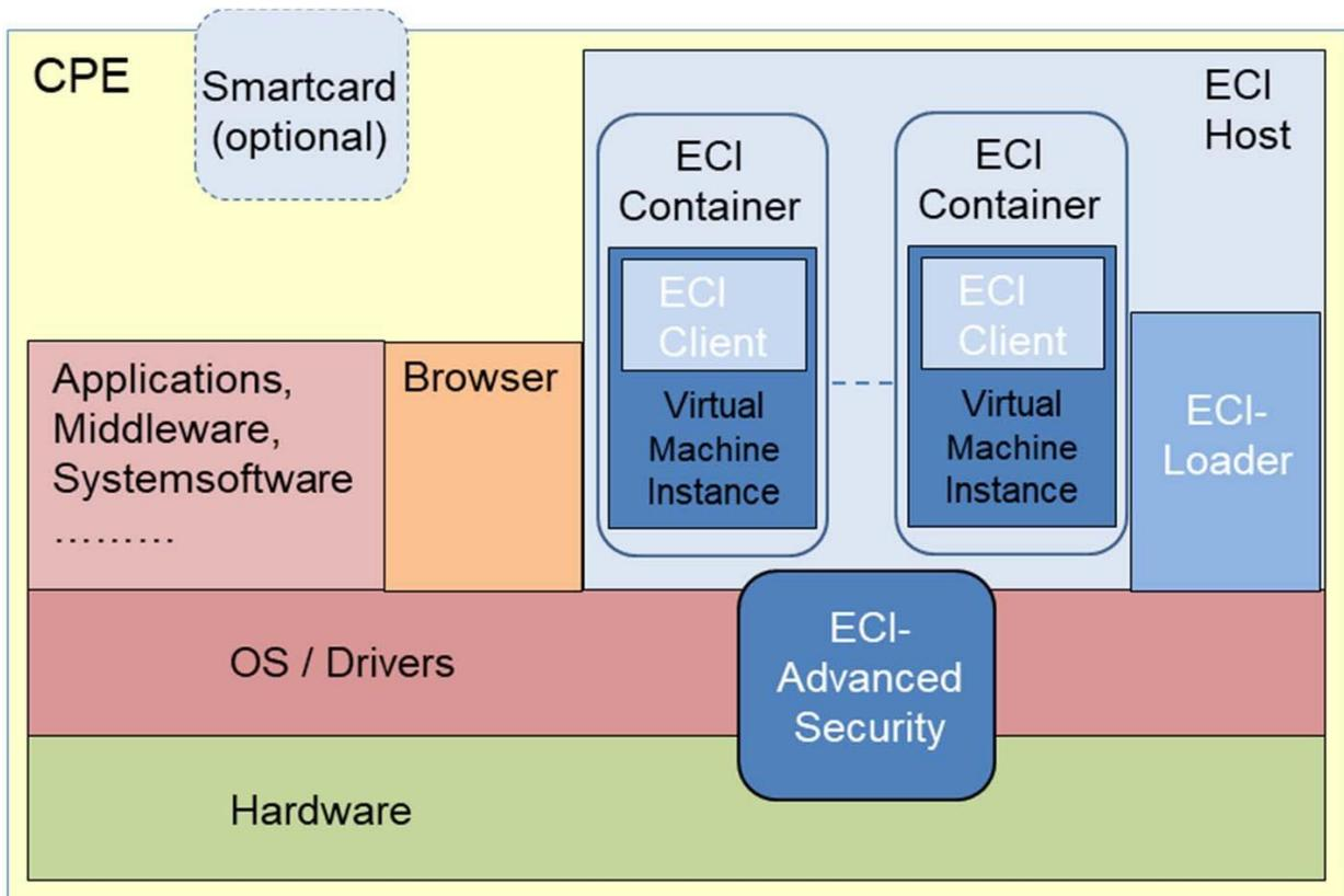
*Figure 13: Block Diagram of CPE as per ECI Standard*
