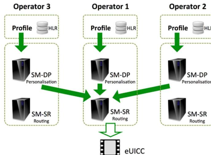
Figure 2.2: Profile interoperability<sup>31</sup> through integration of SM-DP of another operator with the existing SM-SR
