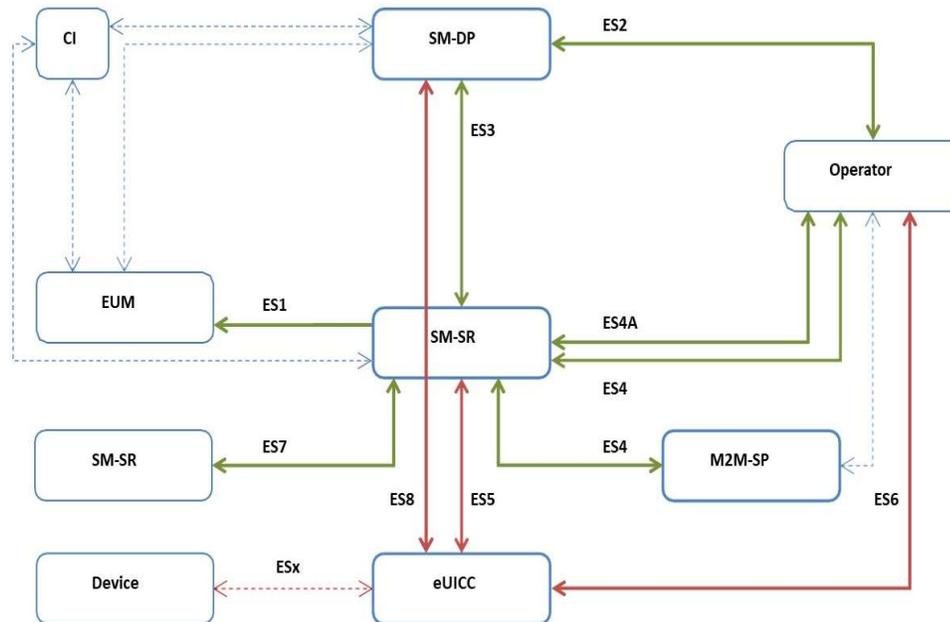
Figure 1.1: Remote Provisioning Architecture for M2M eSIM
