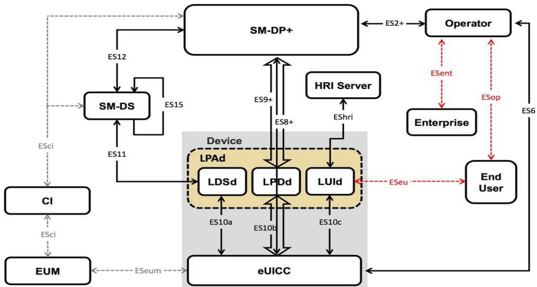
Figure 1.2: Remote SIM Provisioning and Management of the eUICC for Consumer Devices [Source: GSMA SGP.22<sup>7</sup>]
