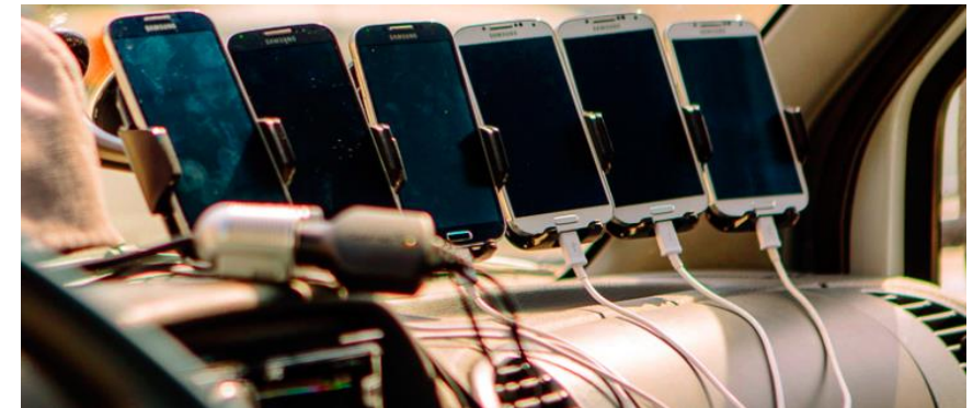
Mobile Internet quality meas. system (Swissqual) 2.800.000 measurements per month
